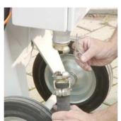
7. connect the air-pressure-hose at the machine.
